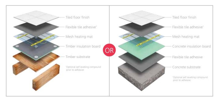
Option 1: Insulating a timber substrate
