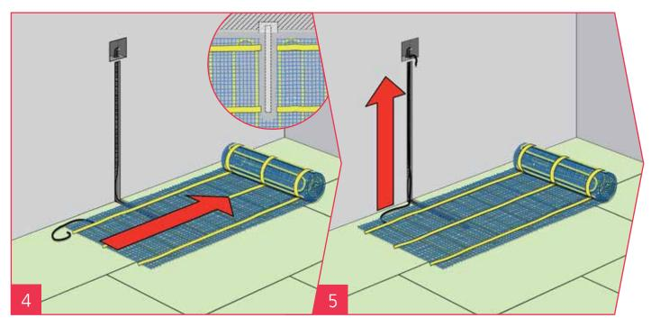
Step 4: Roll out the mesh as planned
